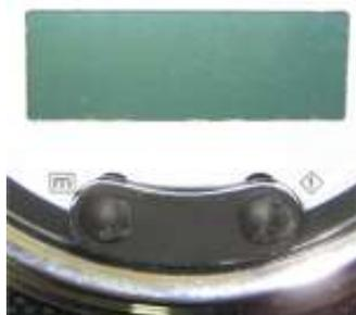
Once in the Settings and Diagnostics menu, pressing the **m** or **t** buttons separately moves the reverse video highlight (**example**) up or down through the list, as indicated by the arrows. The highlighted item is selected when both **m** and **t** buttons are pressed at the same time. If no button is pressed for 5 seconds, the LCD will go back to the standard Drive Screen. The items available in the menu are:
