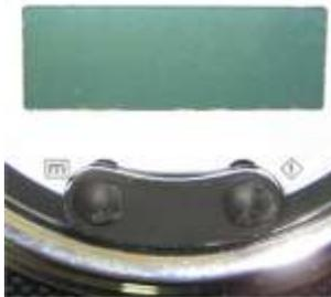
The selected parameter is highlighted with reverse video (**sample**). The selected parameter is retained automatically after 5 seconds of inactivity; no further button presses are required. When the parameter is retained, the reverse video disappears.
