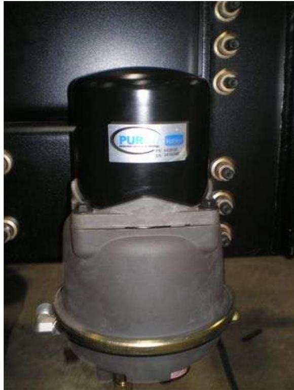
The Tiffin PowerGlide chassis air brake system features a Haldex Purest air dryer which removes the condensed moisture from compressed air. The air dryer is equipped with a desiccant cartridge that needs to be changed every 36 months. The dryer is located on the left hand frame rail (behind the rear axle).
