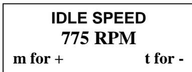
Idle speed is adjusted by using the Set & Resume or by using the message center control switches. The actual engine speed will be displayed as the adjustment is made. Once the Set or Resume switch has been released, there will be a 10 second delay in removing the Idle Speed Adjust screen from the LCD. The new idle speed will be retained in the engine control module as the default setting.
