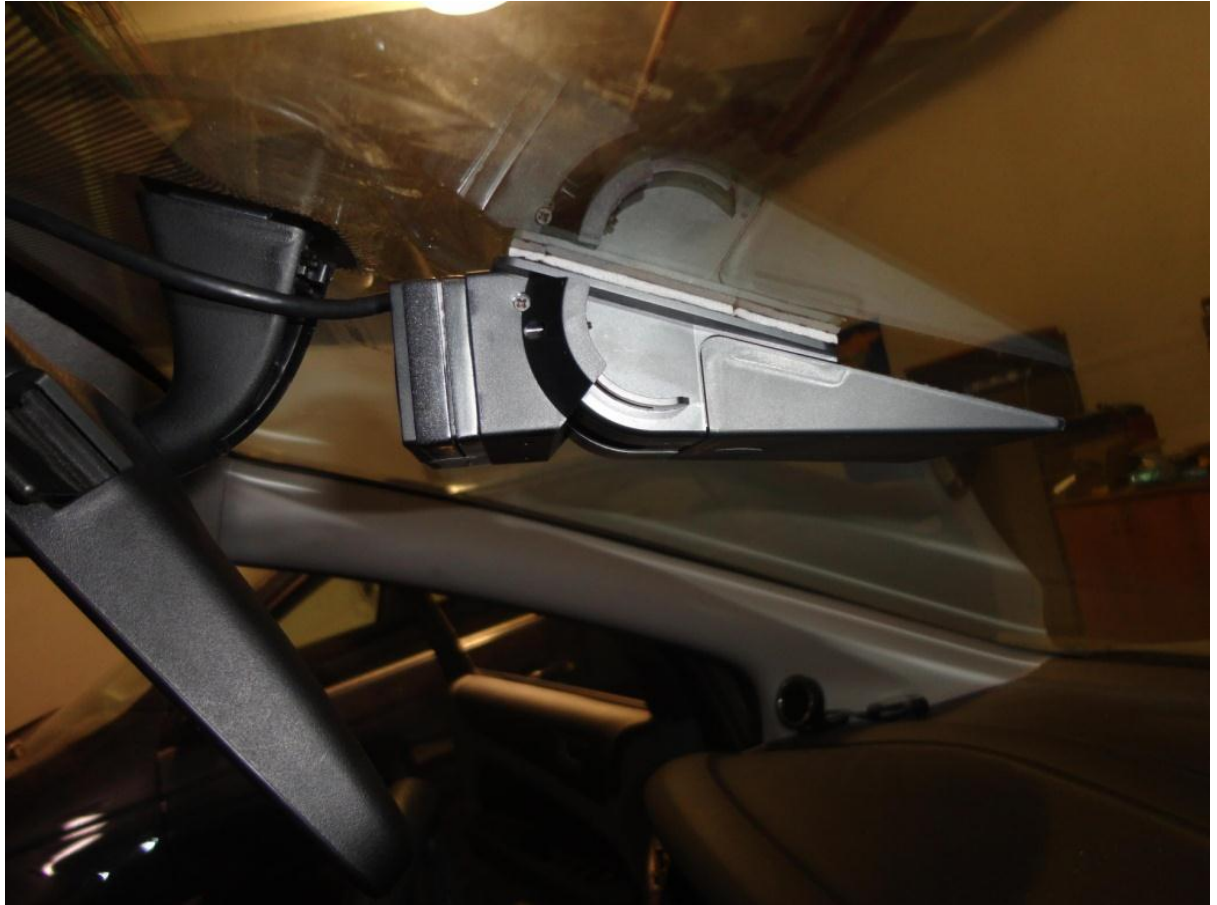
Figure 1-10 Vision Sensor Unit located on the windshield behind the rear view mirror
