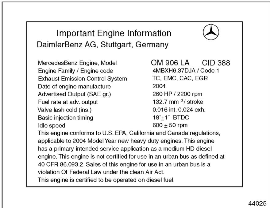
**Figure 1 Emission Label, 6-Cylinder EGR Engine**
