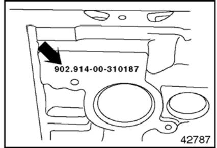
**Figure 12 Engine Identification Number**
