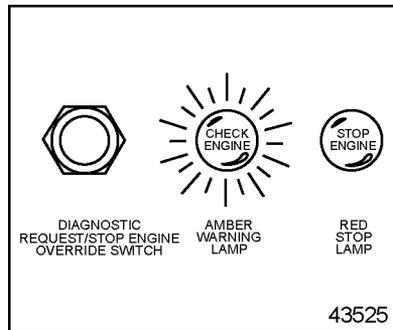
**Figure 26 Typical SEO Switch and Warning Lamps**
