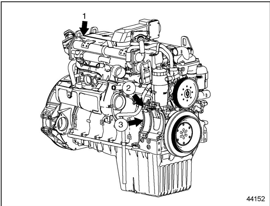
1. Intake Manifold Pressure/Temperature Sensor
