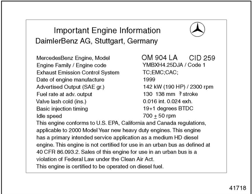
**Figure 4 Emission Label, Non-EGR 4-Cylinder**
