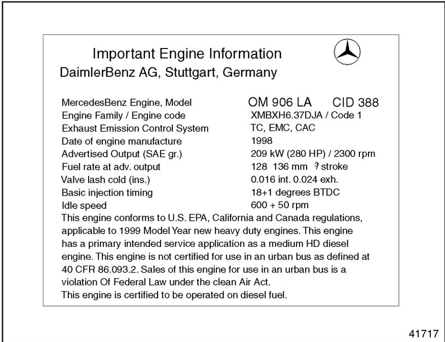
**Figure 3 Emission Label, Non-EGR 6-Cylinder**
