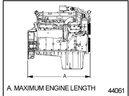
**Figure 29 Engine Measurements (Side View)**
