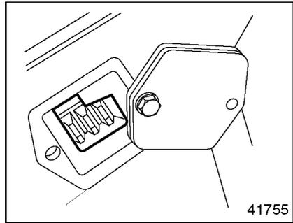
**Figure 35 Inspection Hole in the Timing Case**
