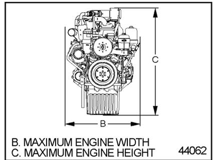
**Figure 30 Engine Measurements (Front View)**
