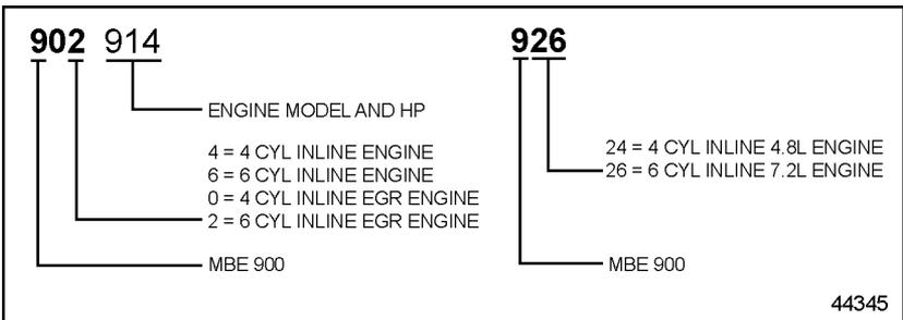
**Figure 13 Engine Identification**
