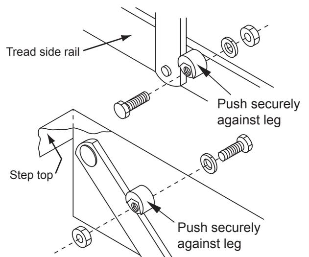
**WARNING:** When the cam stops are out of adjustment, the step may feel loose or 'mushy' when stepped on. If the cam stops are not properly adjusted the step may not extend fully to the locked-out position. Using a step with loose or out-of-adjustment cam stops may cause damage to the motor assembly and/or the drive linkage.
