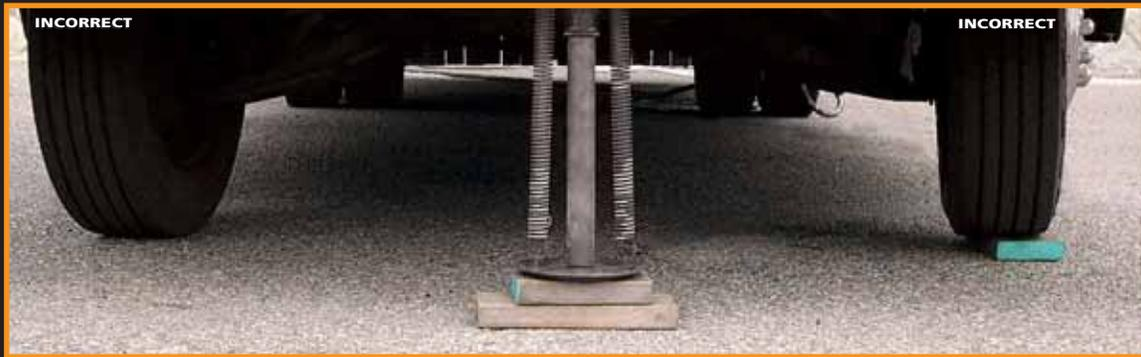
The correct and incorrect methods are shown below. Note in the correct method, the blocks are wider than the tread and longer than the tire's footprint. This provides maximum support to the tires and assures that the load is evenly distributed.
