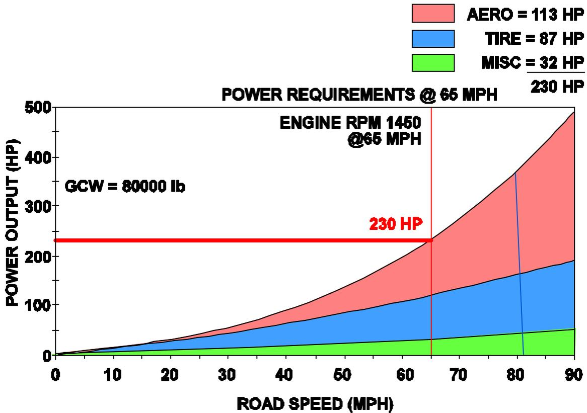
Notice that these aerodynamic treatments are more effective at higher speeds and the power required to overcome things like tire rolling resistance are not affected by the aerodynamic aids.
