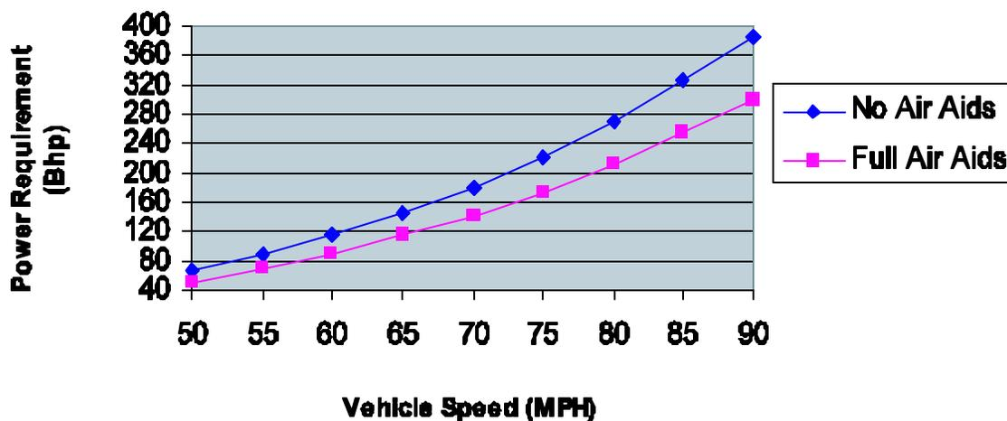
At approximately 0.3 lb./BhpHr fuel consumption, a reduction of 35 Bhp required to cruise at 65 mph results in a savings of about 10.5 lbs. of fuel every hour ( $0.3 \times 35 = 10.5$ ). Since diesel fuel weighs about 7.1 lb./gal., this amounts to a savings of 1.5 gallons of fuel saved every hour ( $10.5/7.1 = 1.5$ ). For a truck running 10 hours per day, that's 15 gallons of fuel saved per day. At \$1.50 per gallon of fuel, the dollar savings is \$22.50 per truck per day.
